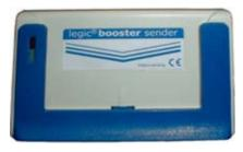
The onboard mobile Legic long-range booster sender reads the data of an inserted Legic-badge card and after a button press, stores and analyses the data.
